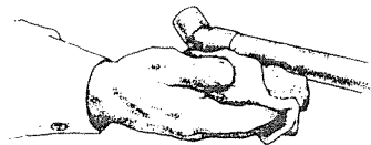
7. Remove excess solder with a small brush or wiping cloth while plastic, leaving a fillet around end of fitting as it cools.
