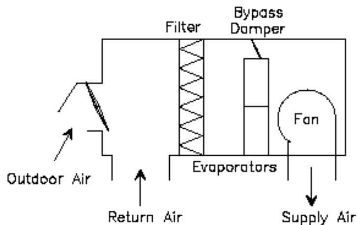
Figure 7.4 - Schematic of DX System with Two-Position Bypass Damper
