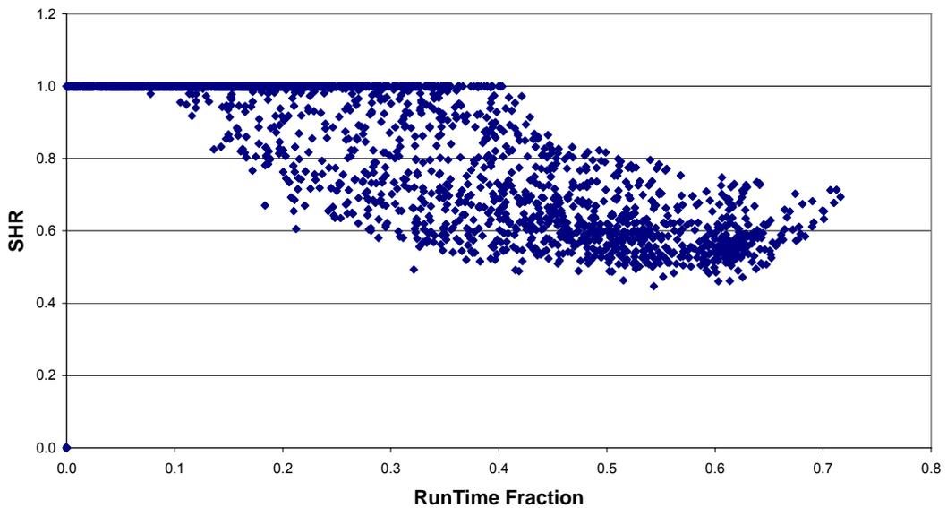
**Figure 9.5 Sensible Heat Ratio (SHR) vs. Runtime Fraction With Latent Degradation.**
