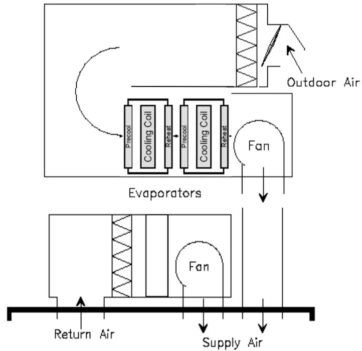
**Figure 7.10 - Schematic of Dual Path System with AAHX**
