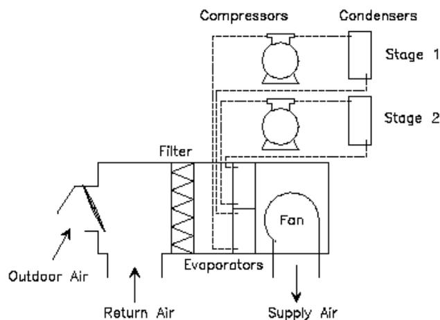
**Figure 7.1 - Schematic of DX RTU**
