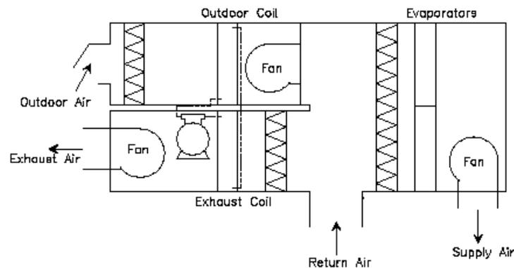
**Figure 7.7 - Schematic of DX System with Outdoor Air Preconditioning**
