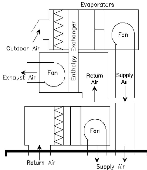
**Figure 7.9 - Schematic of Dual Path System with Enthalpy Recovery**
