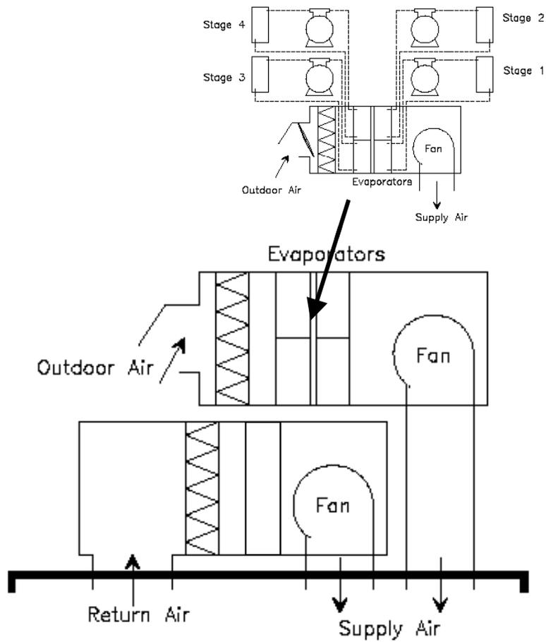
**Figure 7.8 - Schematic of Dual Path System**
