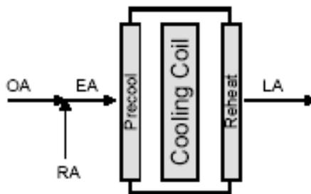
Figure 7.2 - Schematic of DX Cooling Coil with Air-to-Air Heat Exchanger
