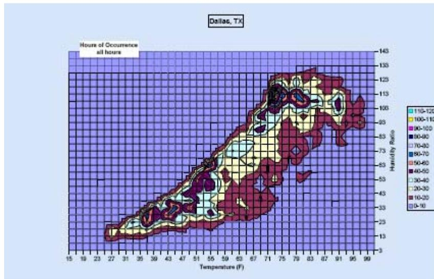
Figure 4.5 - Joint Frequency Chart for Dallas, TX TMY2 Weather Data
