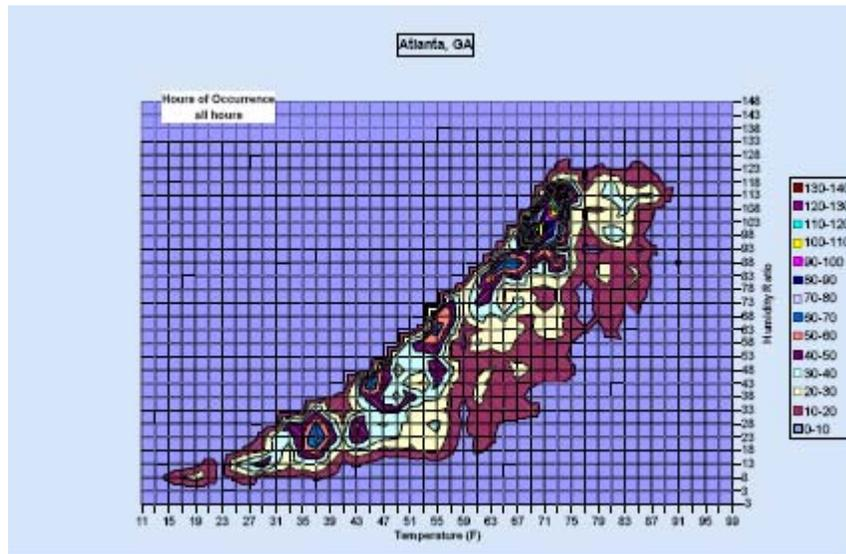
**Figure 4.7 - Joint Frequency Chart for Atlanta, GA TMY2 Weather Data**
