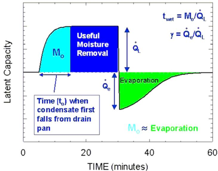
**Figure 9.3 Concepts of Moisture Buildup and Evaporation**
