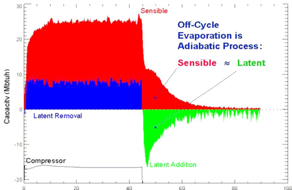
**Figure 9.1** Transient Sensible and Latent Capacity of a Cooling Coil Over an Operating Cycle
