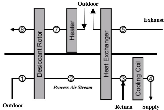
**Figure 7.5 - Schematic of Hybrid Integrated Desiccant and DX System**
