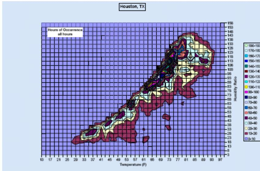
Figure 4.4 - Joint Frequency Chart for Houston, TX TMY2 Weather Data
