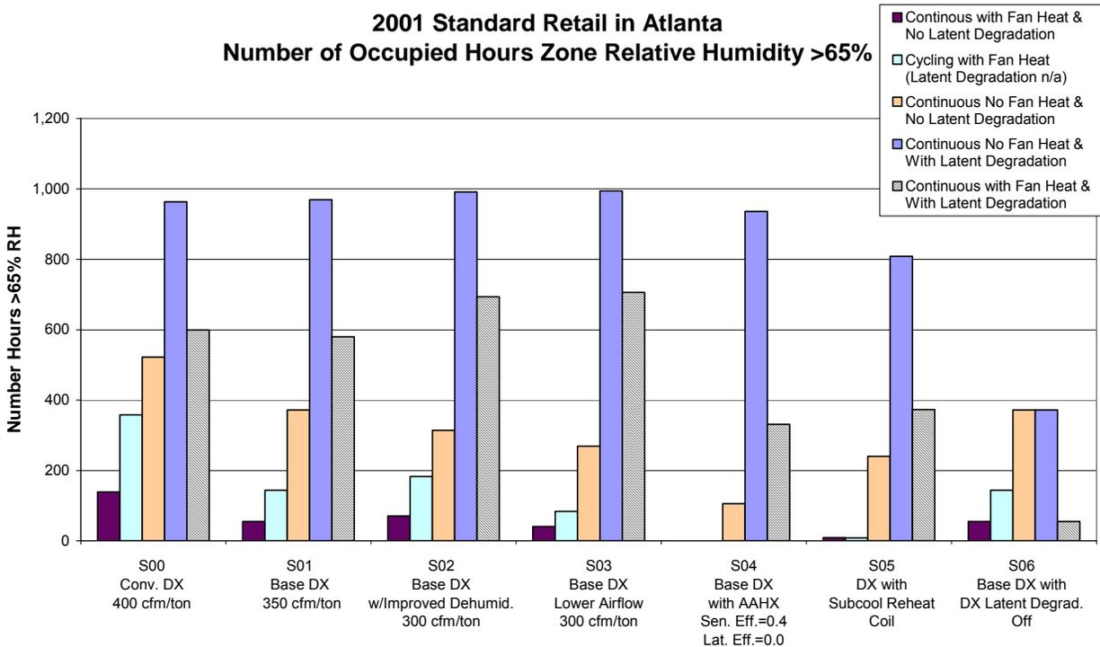
**Figure 12.5 Impact of Fan Heat and Latent Degradation on Humidity Control.**
