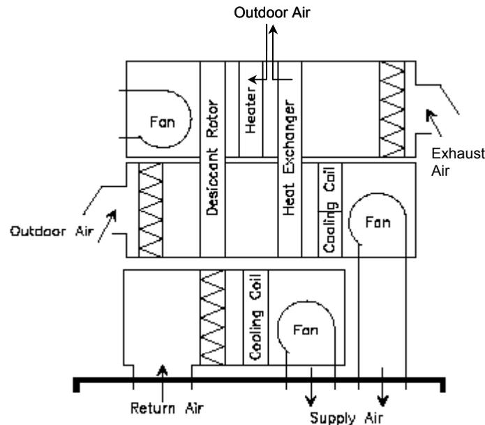
Figure 7.11 – Hybrid DX/Desiccant Dual Path System
