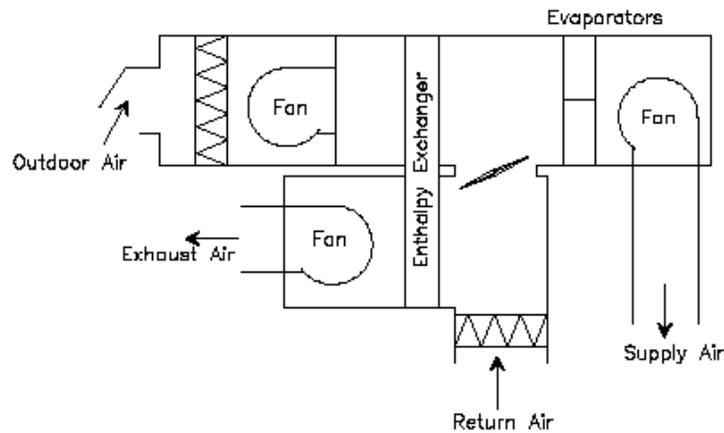
**Figure 7.6 - Schematic of Enthalpy Recovery in DX System**
