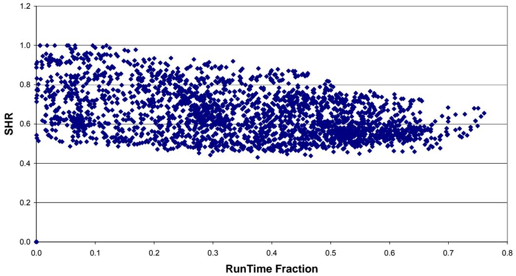
**Figure 9.4 Sensible Heat Ratio (SHR) vs. Runtime Fraction With No Latent Degradation.**
