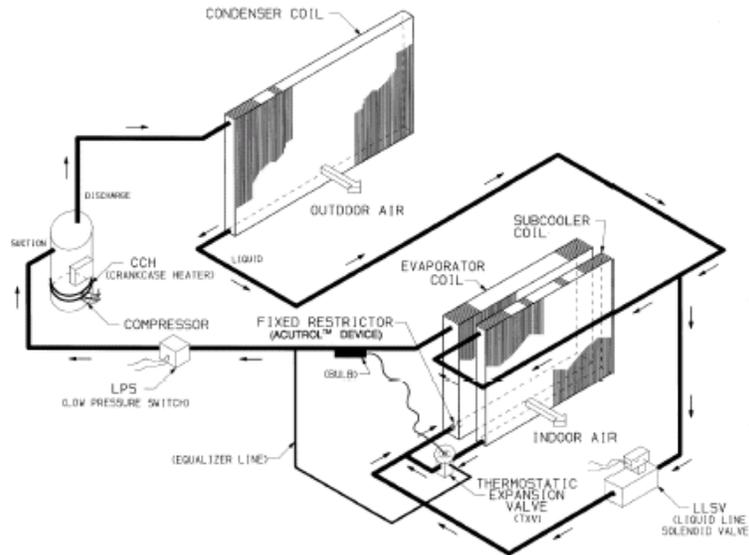
**Figure 7.3 - Schematic of DX System with MoistureMiser (from Carrier)**
