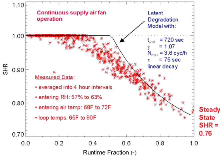
**Figure 9.2 Field Data Showing the Net Impact of Part-Load Operation on Sensible Heat Ratio**
