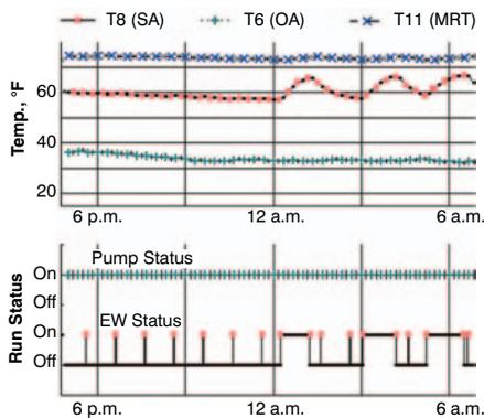
**Figure 5:** Trend plot of DOAS supply air temperature (T8) with panel pump on.
