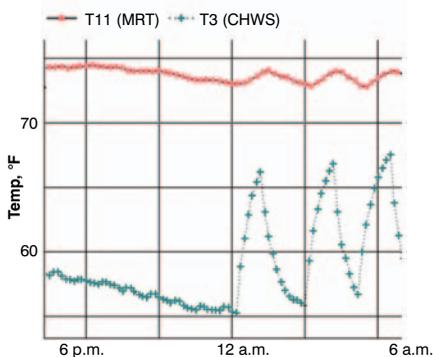
**Figure 8:** Trend plot of panel inlet water temperature (T3) with panel pump on.
