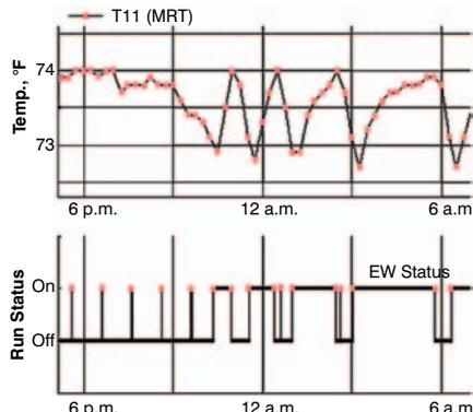
**Figure 3: Trend plot of space temperature (T11) with panel pump off.**
