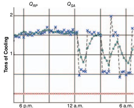
**Figure 7:** Trend plot of DOAS cooling parameters ( $Q_{SA}$ ,  $Q_{RP}$ ) with panel pump on.
