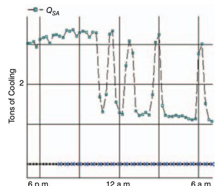
**Figure 4: Trend plot of DOAS cooling parameters ( $Q_{SA}$ ) with panel pump off.**
