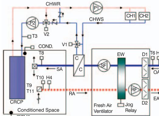
**Figure 1: Schematic of the system used for field tests. The building houses architecture students.**
