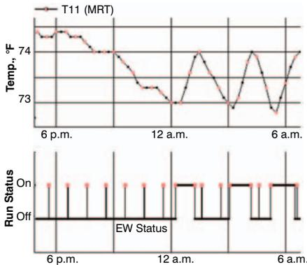
**Figure 6:** Trend plot of space temperature (T11) with panel pump on.
