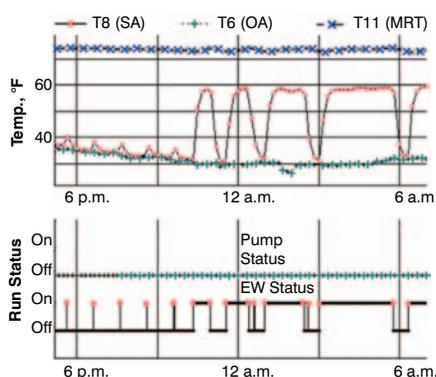
**Figure 2: Trend plot of DOAS supply air temperature (T8) with panel pump off.**
